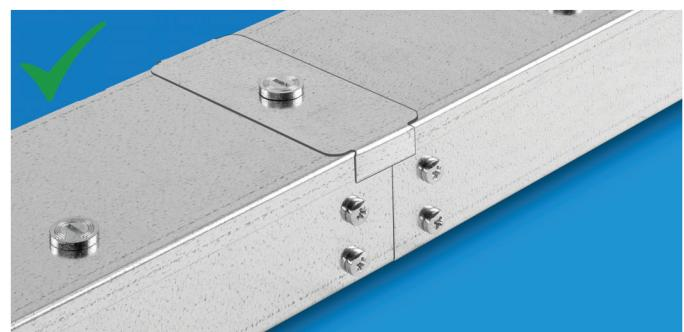
The lid joint on the left is again non-compliant. A cover strap is therefore required to keep the IP4X integrity on the length lid. This can be fixed anywhere along the length and does not require alignment with the coupler and screw heads.
